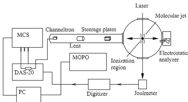
FIG. 1. Schematic diagram of the TOF spectrometer.
