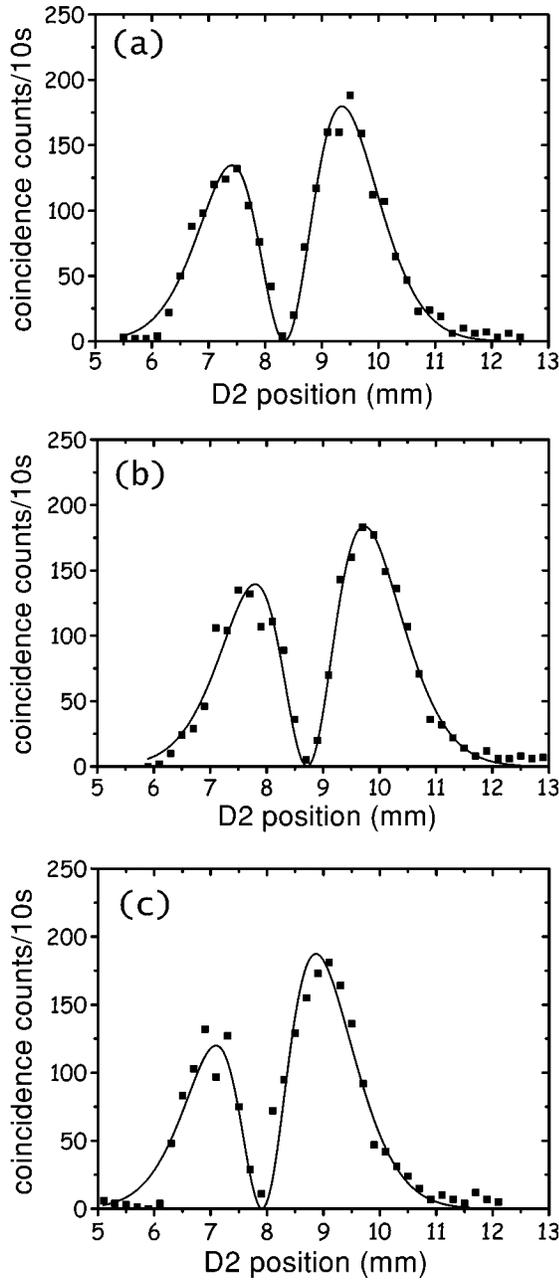
FIG. 4. Coincidence profile scanning D2 with D1 fixed. (a) D1 at the minimum of the profile in Fig. 3; (b) D1 displaced by +0.4 mm; and (c) D1 displaced -0.4 mm.
