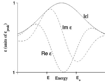
FIG. 4. The light pulse (in frequency space) used to excite the Autler-Townes split  $|2P_0\rangle$  state from the ground  $1S$  state to produce the optimal  $c_{\alpha}$  coefficients. This choice of coefficients is the one most effective in delaying the emission (in the absence of the interruptions) over the optimization time of 2.4 ns.
