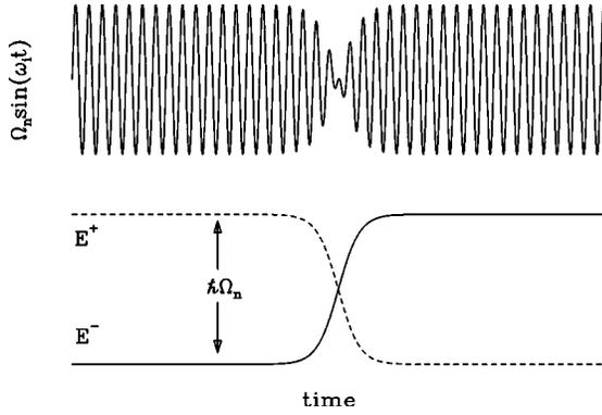
FIG. 6. The train wave of the spectator cw field of frequency  $\omega_i$  near an interruption which switches  $\Omega_{n_i}$  to  $-\Omega_{n_i}$ , thereby exchanging the order of the  $E_{n_i}^{\pm}$  levels, as shown in the lower panel.
