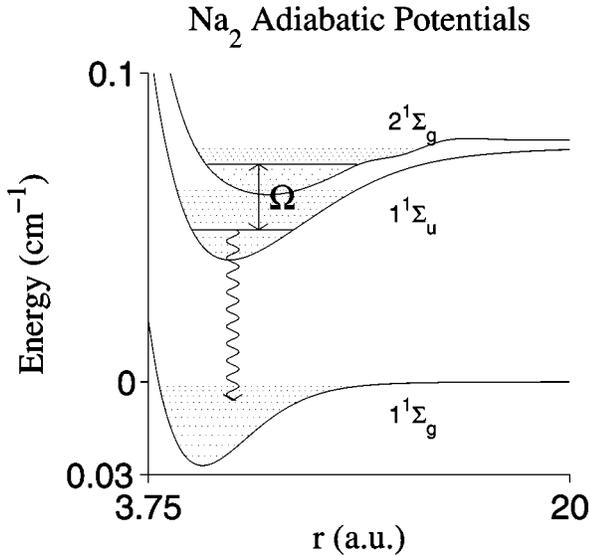
FIG. 8. The three lowest singlet potential-energy curves of  $\text{Na}_2$ :  $1^1\Sigma_g$ ,  $1^1\Sigma_u$ , and  $2^1\Sigma_g$ . Every fifth vibrational level is marked with a dashed line. The  $|a\rangle$  state is the  $\nu=20$  vibrational level of the second potential. The  $|b\rangle$  state is the  $\nu'=30$  vibrational level of the third potential. Both are marked by solid lines. The Franck-Condon factor (equal to overlap integral) between these two states is 0.118.
