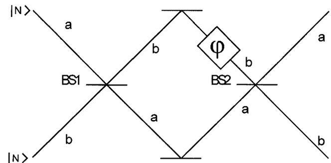
FIG. 1. Schematic of the Mach-Zehnder interferometer for the detection of the phase difference  $\varphi$  when the twin Fock states  $|N\rangle_a|N\rangle_b$  are injected into the first beam splitter.
