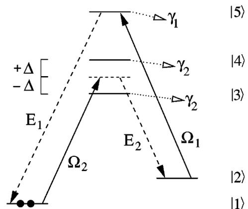
FIG. 1. Four-wave mixing in a modified double- $\Lambda$  system with  $\text{sgn}(d_{42}/d_{41}) = -\text{sgn}(d_{32}/d_{31})$ , with  $d_{ij}$  being the dipole moment of the  $|i\rangle - |j\rangle$  transition.
