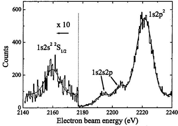
FIG. 4. A portion of the “ $K_\alpha$  cut” projection (horizontal) from the Fig. 3 scatter plot is shown, highlighting the He-like part of the KLL DR events’ x-ray intensity as a function of the electron-beam energy.
