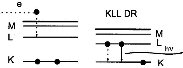
FIG. 1. Illustration of KLL dielectronic recombination for a He-like ion. Both electrons in the doubly excited intermediate state have the possibility to relax into the 1s shell.
