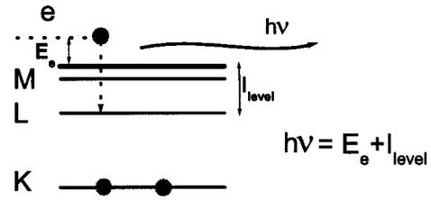
FIG. 2. Illustration of  $n=2$  radiative recombination for a He-like ion.
