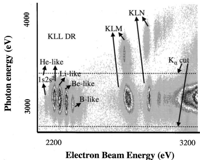
FIG. 3. Scatter plot of the x-ray intensity vs the electron-beam energy (X axis) and x-ray energy (Y axis). The first group of spots is the KLL DR resonances to the He-like, Li-like, Be-like, and B-like Ar ions. The KLM, KLN, and other DR events can be seen in the figure. Taking the “ $K_\alpha$  cut” produces the spectrum shown in Fig. 4.
