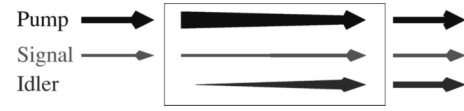
FIG. 2. NPA, nondegenerate parametric amplification. The thickness of the arrows is intended to give an indication of how the energy of the field components changes during propagation through the crystal.
