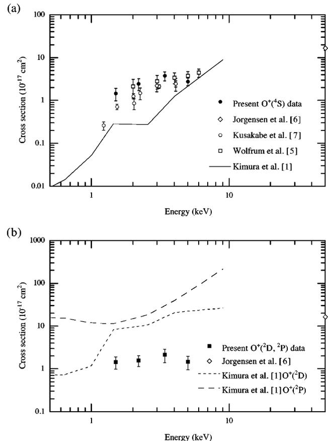
FIG. 3.  $O^+$ -He total charge-transfer cross sections: (a)  $O^+(^4S)$ -He and (b)  $O^+(^2D, ^2P)$ -He. Note that only the lowest-energy measurement of Jorgensen *et al.* [6] is shown.
