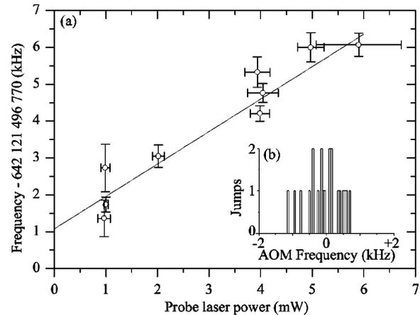
FIG. 3. (a) Frequency of the octupole transition as a function of probe laser power. (b) The spectrum of a single scan of the octupole transition, prior to combination with femtosecond comb data.
