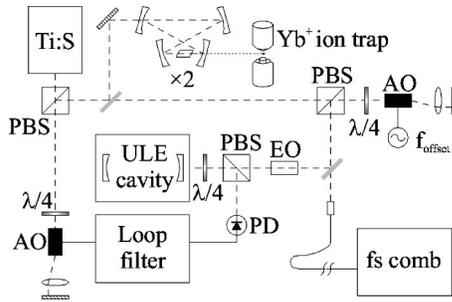
FIG. 2. Schematic of the probe laser system. EO, electro-optic modulator; AO, acousto-optic modulator; PD, photodiode, PBS, polarising beam splitter.
