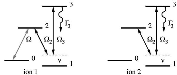
FIG. 3. Level scheme of a dissipation-assisted phase gate with cold trapped ions. In addition to the basic setup shown in Fig. 1, a strong laser field couples the state  $|1\rangle$  with detuning  $\nu$  to an auxiliary atomic state  $|3\rangle$ . Populating this level leads to the emission of photons with a rate  $\Gamma_3$ .
