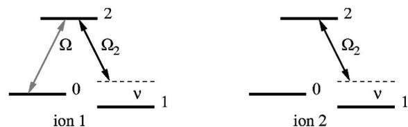
FIG. 1. Level scheme for implementation of a phase gate. A strong laser field with detuning  $\nu$  establishes coupling between the ions via a common vibrational mode. In addition, a laser pulse individually addressing the 0-2 transition of ion 1 is required.
