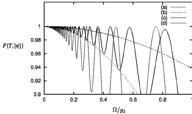
FIG. 2. The fidelity of a single phase gate as a function of  $\Omega/g_2$  for the initial qubit states  $|00\rangle$  (a), (b) and  $|01\rangle$  (c), (d). The curves (a), (c) result from an exact solution of the time evolution (1) while the curves (b), (d) result from Eq. (5).
