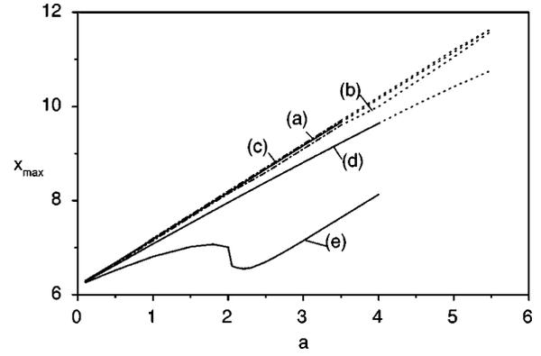
FIG. 2. Position of the peak of the wave function  $x_{\max}$  versus the barrier width  $a$  at  $t=0.1$  for  $p_0=146$ ,  $V_0/m_0c^2=1.5$ , and  $\Delta p_0=(a)0.5$ , (b) 2.0 (dashed lines), and  $V_0/m_0c^2=2.2$  with  $\Delta p_0=(c)0.5$ , (d) 2, and (e) 3.5 (solid lines). The dotted parts of the lines correspond to situations where the average values are superluminal.
