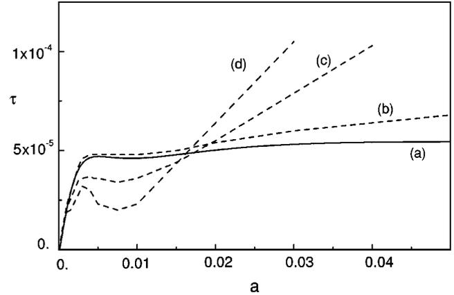
FIG. 7. Curve (a): Hartman phase time  $\tau_H$  versus  $a$  for  $E/m_0c^2=1.46$  and  $V_0/m_0c^2=2.2$ . Traversal time  $\tau_{tr}$  versus  $a$  for  $\Delta p_0=2$  [curve (b)],  $5$  [curve (c)], and  $8$  [curve (d)].
