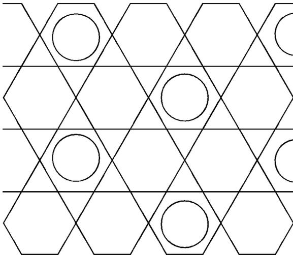
FIG. 4. Kagomé lattice with  $N$  spins. The circles mark the  $N/9$  hexagons in which independent magnons can be localized.
