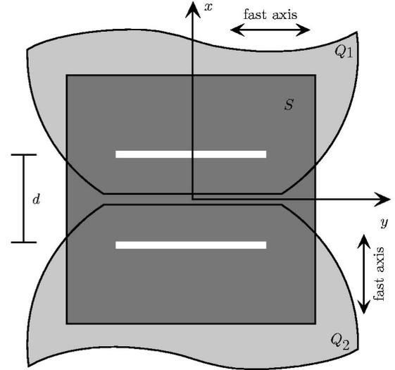
FIG. 3. The birefringent double slit. The quarter wave plates  $Q_1$  and  $Q_2$  are aligned with orthogonal fast axes.  $S$  is a double slit with slit separation  $2b$ .
