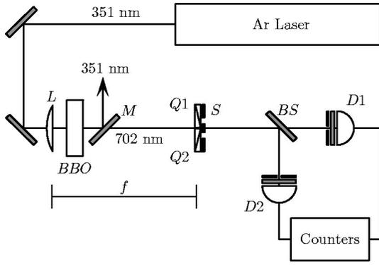
FIG. 1. Schematic diagram of spatial antibunching setup. An Ar laser pumps a BBO crystal, generating correlated photons. The down-converted photons are incident on the birefringent double slit  $S$  and then the beam splitter  $BS$ . The pump beam is focused on the double slit. Single and coincidence counts are registered with detectors  $D_1$  and  $D_2$ .
