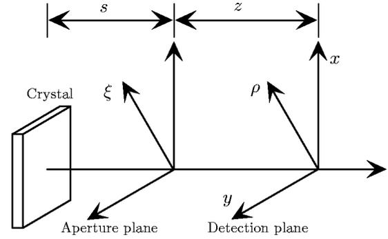
FIG. 2. Illustration of the geometry.  $s$  is the crystal-aperture distance and  $z$  is the aperture-detector distance.
