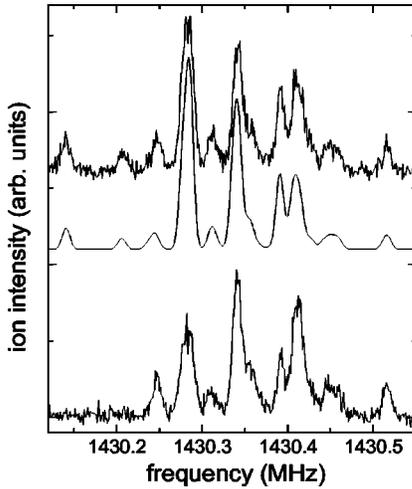
FIG. 7. High-resolution pure inversion spectra of  $^{15}\text{ND}_3$  ( $|J,K\rangle=|1,1\rangle$ ), measured by probing the lower inversion level. The upper experimental spectrum is recorded while operating the hexapole in the pulsed mode, and is shown together with the theoretical spectrum obtained from the best fit to the experimental data. The lower experimental spectrum is recorded when the molecules leave the hexapole adiabatically.
