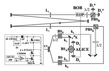
FIG. 1. Experimental apparatus realizing the "active" quantum state teleportation protocol (QST). The cross close to the center of the optical delay line indicates the approximate position of the focal region of the lens  $L_1$ . Inset: Diagram of the fast electronic switch of the electro-optic Pockels cell (EOP) implementing the unitary transformation:  $U \equiv \sigma_z$ .
