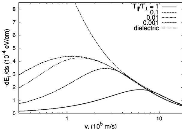
FIG. 12. Energy loss of protons in the present binary collision model for increasing asymmetry  $T_\perp/T_\parallel$  of the velocity distribution and in the dielectric theory with a flat velocity distribution,  $T_\parallel=0$  [9]. Standard parameters of Ref. [9]:  $n_e=3 \times 10^{14} \text{ m}^{-3}$ ,  $k_B T_\perp=1 \text{ eV}$ ,  $B=0.07 \text{ T}$ .
