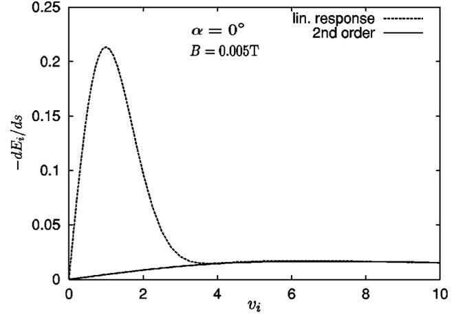
FIG. 4. Energy loss in units of  $4\pi(Z\ell^2)^2 n_e / (mv_{\text{th}\parallel}^2)$  as a function of the ion velocity  $v_i$  in units of the longitudinal thermal velocity  $v_{\text{th}\parallel}$  for  $B=5$  mT and  $\alpha=0^\circ$ . Other parameters are from Table I. Solid curve: present second-order treatment; dashed curve: linear-response theory [22].
