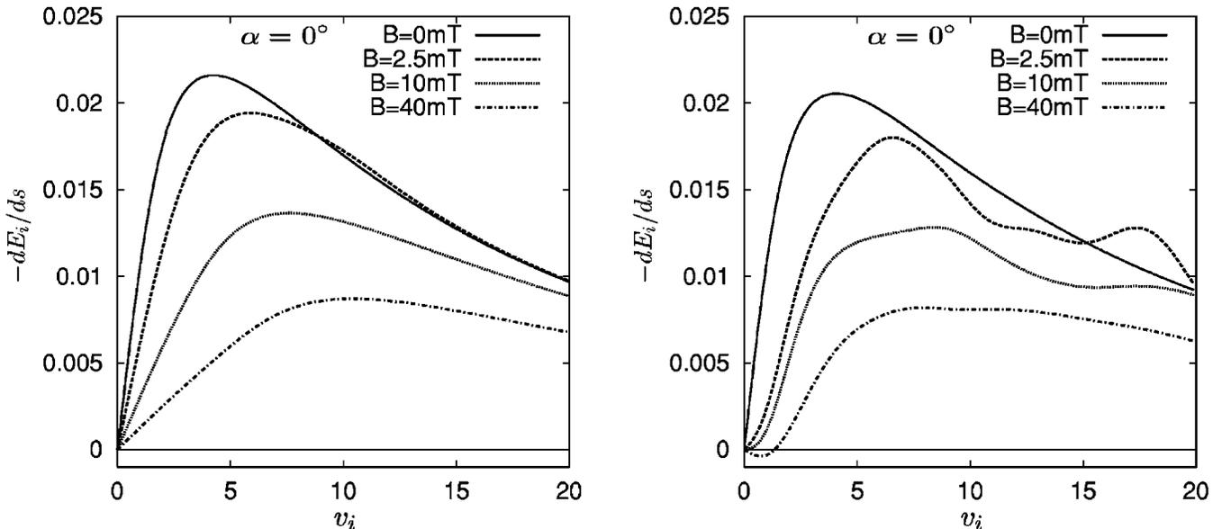
FIG. 8. Energy loss in units of  $4\pi(Ze^2)^2 n_e / (mv_{\text{thll}}^2)$  as a function of the ion velocity  $v_i$  in units of the longitudinal thermal velocity  $v_{\text{thll}}$  for  $\alpha = 0^\circ$  and various magnetic-field strengths. Other parameters from Table I. Left panel: present second-order theory; right panel: CTMC results [3-5].
