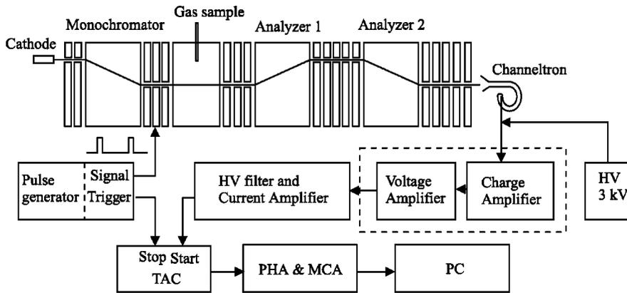
FIG. 1. Schematic diagram of the spectrometer including electronic circuits of the time-of-flight resolved measurements.
