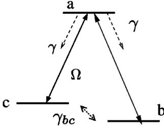
FIG. 1. Three-level model scheme. The upper level  $a$  decays to  $b$  and  $c$  with decay rate  $\gamma$ . The relaxation rate between levels  $b$  and  $c$  is denoted as  $\gamma_{bc}$ , which is assumed to be small compared to  $\gamma$ .
