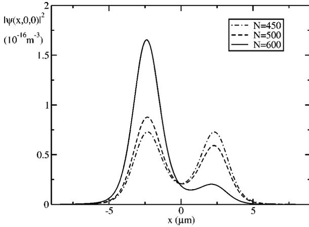
FIG. 1. Density distribution of the lithium BEC in real space for  $N=450$  (dashed-dot line),  $N=500$  (dashed line), and  $N=600$  (solid line) with  $A_n \equiv A/\hbar = 2650 \text{ s}^{-1}$  and  $\sigma = 5 \text{ }\mu\text{m}$ .
