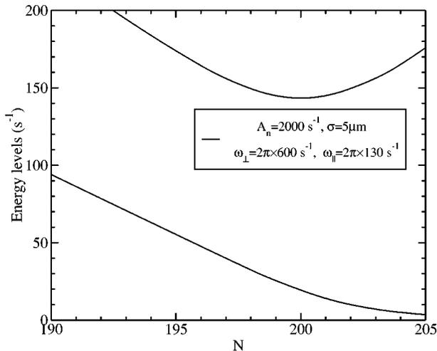
FIG. 4. First two excited energy levels versus the number of atoms  $N$ . The system parameters are  $\omega_{\perp} = 2\pi \times 600 \text{ s}^{-1}$ ,  $\omega_{\parallel} = 2\pi \times 130 \text{ s}^{-1}$ ,  $A_n \equiv A/\hbar = 2000 \text{ s}^{-1}$ , and  $\sigma = 5 \mu\text{m}$ .
