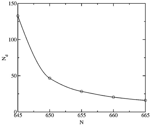
FIG. 8. Number  $N_d$  of lost atoms for which the coherence decays by  $1/e$  versus the total number of atoms, for  $A_n \equiv A/\hbar = 2000 \text{ s}^{-1}$  and  $\sigma = 5 \text{ }\mu\text{m}$ .
