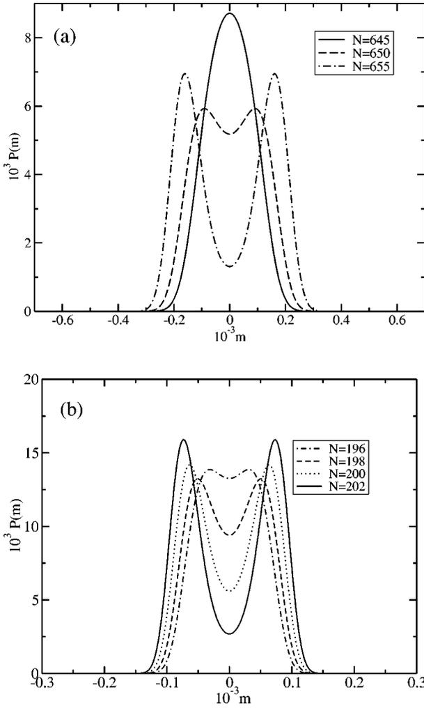
FIG. 6. Probability distribution of the “barycenter” indicator for the lithium BEC, for different  $N$  values and for a standing wave with  $A_n = 2000 \text{ s}^{-1}$  and  $\sigma = 5 \text{ }\mu\text{m}$ ; (a)  $\omega_{\perp} = 2\pi \times 150 \text{ s}^{-1}$  and (b)  $\omega_{\perp} = 2\pi \times 600 \text{ s}^{-1}$ .
