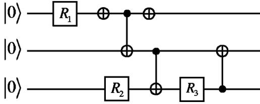
FIG. 3. Quantum logic circuit for preparation of the  $W$  state from direct product state  $|0\rangle|0\rangle|0\rangle$ . The denotations are the same as in Ref. [15].
