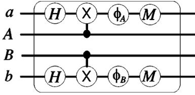
FIG. 4. Quantum circuit of the purification protocol. This circuit consists of local operations at different nodes of the quantum network, where  $H$  denotes a Hadamard transformation, which is followed by a controlled-NOT gate, with the cavity field and atom as source and target, respectively. There is a phase gate, which allows rotating the atomic state in a given angle  $\phi$ . Finally, we have included the measurement on the ancillary system.
