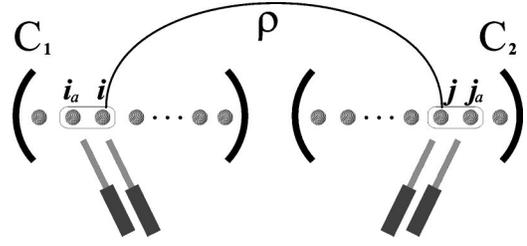
FIG. 7. Setup for purification protocol using trapped ions inside an optical cavity. The entanglement between ions  $i$  and  $j$  is purified by local operations on pairs  $(i, i_a)$  and  $(j, j_a)$ .
