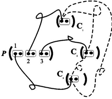
FIG. 8. Diagram for establishing multiparticle entanglement. Initially ions in the central cavity  $P$  are entangled with ions in cavities  $C_j$ . The initial entanglement is described with solid lines. After a collective measurement in cavity  $P$  on ions 1, 2, and 3 a maximally entangled state among cavities  $C_1$ ,  $C_2$ , and  $C_3$  is achieved.
