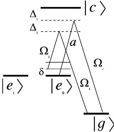
FIG. 6. Electronic structure of trapped ions in a linear trap inside the cavity.
