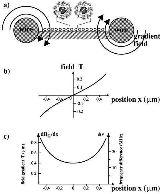
FIG. 1. (a) Arrangement of wires that generate the magnetic field gradient. The currents  $I$  in the two wires are equal and parallel. (b) Field distribution along the chain of the qubits for a separation of  $\Delta=1 \mu\text{m}$  and  $I=1 \text{ A}$ . (c) Corresponding field gradient. The vertical axis also indicates the frequency separation between neighboring electron spins, for a separation of  $1.14 \text{ nm}$ .
