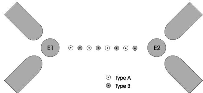
FIG. 4. Diagram showing how the confined ammonia molecules could be used in a cellular automaton approach.
