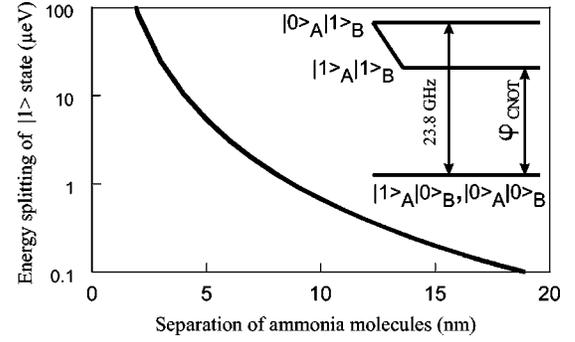
FIG. 2. Diagram showing the energy-level splitting of an ammonia molecule  $A$  due to the presence of adjacent ammonia  $B$ . A desirable, 1%, splitting of about  $1 \mu\text{eV}$  corresponds to a separation of 9 nm (approximately the resolution of fabrication by electron-beam lithography). The inset shows the energy-level diagram, the splitting corresponding to that of the  $|1\rangle_B$  levels.
