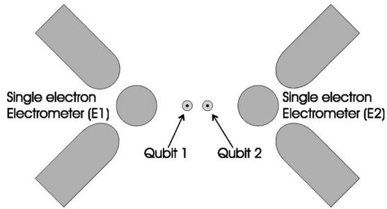
FIG. 3. Schematic illustration of a two-qubit geometry with two single-electron electrometers and a gate. The gate should not be confused with the  $J$  gate in the Kane model: it doesn't turn the interaction on and off but, together with the floating electrometers, tunes the individual qubits.
