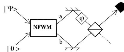
FIG. 1. Modified Mach-Zehnder interferometer where the first beam splitter has been replaced by a nonlinear four-wave mixer operating under the conditions required to produce maximally entangled states for an even input state  $|\Psi\rangle$ . Detection is performed only on the output  $b$  mode.
