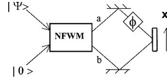
FIG. 4. Using the nonlinear four-wave mixer for photolithography. Here  $\phi = 2\pi x/\lambda$  where  $x$  represents the lateral position across the substrate. The substrate is assumed to absorb an even number  $N$  of photons.
