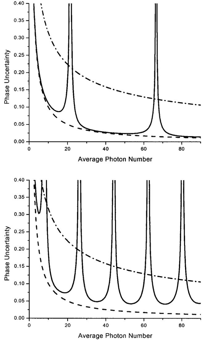
FIG. 2. Phase uncertainty  $\Delta\varphi$  versus average photon number  $\bar{n}$  for the input even coherent states (solid line) for the phase difference (a)  $\varphi = \pi/45$  and (b)  $\varphi = \pi/18$ . The dashed lines represent the Heisenberg limit  $1/\bar{n}$  while the dot-dashed lines represent the standard quantum limit  $1/\sqrt{\bar{n}}$ .
