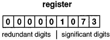
FIG. 4. Realizing variable-length messages by neutral-prefix code words.
