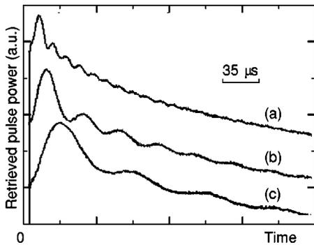
FIG. 5. Time dependence of the beat note power of the retrieved and reading pulses for various values of the magnetic field: (a)  $B = 56$  mG, the oscillation period is  $T_a = 12.6 \mu\text{s}$ ; (b)  $B = 21$  mG, the oscillation period is  $T_b = 34.8 \mu\text{s}$ ; (c)  $B = 10$  mG, the oscillation period is  $T_c = 68.8 \mu\text{s}$ .
