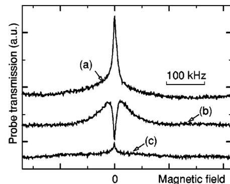
FIG. 11. Transmission of cw probe-laser radiation resonant with the D1 line of  $^{87}\text{Rb}$  vs magnetic field for the atomic cell containing 0.3 Torr of Ne buffer gas. The magnetic field is shown in frequency units as per Fig. 9. The probe and drive beams are spatially separated (the separation is equal to 5 mm). (a) The polarizations of the probe and drive fields are the same. (b) The angle between the polarizations is equal to  $90^\circ$ . (c) The drive field is absent.
