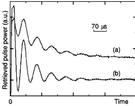
FIG. 8. Time dependence of the beat note power of the retrieved and reading pulses for spatially separated (2 mm) writing and reading beams [curve (a)], and overlapping writing and reading beams [curve (b)]. The maximum of the scattering efficiency shifts in time for the separated beams compared with the overlapping beams.
