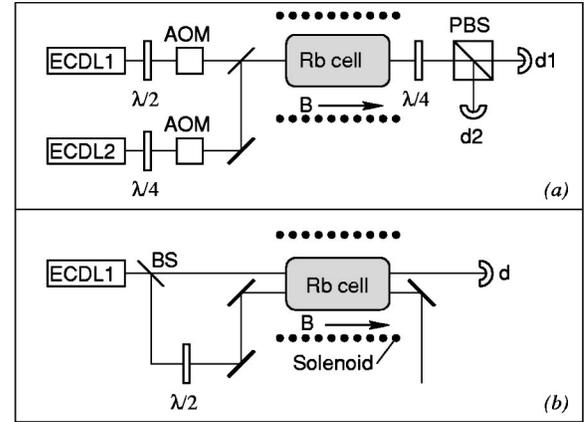
FIG. 1. Experimental setups used for observation of the Ramsey effect in (a) time (pulse regime) and (b) frequency (cw regime) domains.
