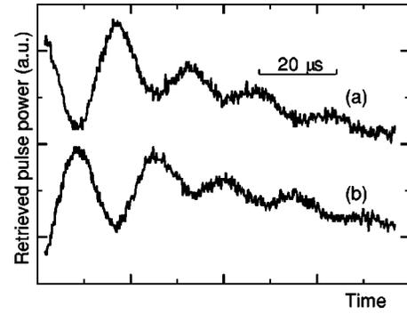
FIG. 6. Time dependence of the beat note power of the retrieved and reading pulses for various polarization directions of the writing fields. The  $45^\circ$  rotation of  $\lambda/2$  plate [see Fig. 1(a)] leads to the  $180^\circ$  phase shift of the oscillations of the power of the retrieved radiation [compare curves (a) and (b)].
