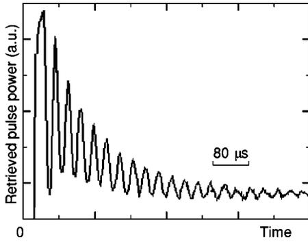
FIG. 4. Time dependence of the beat note power of the retrieved and reading pulses for the magnetic-field  $B = 23$  mG. The origin of the time scale corresponds to the back edge of the writing pulses. The front edges of reading and retrieved pulses coincide.
