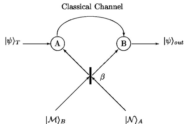
FIG. 1. Schematic experimental setup for teleportation protocol.  $|\mathcal{M}\rangle_B$  and  $|\mathcal{N}\rangle_A$  are input Fock states to a beam splitter of transmissivity  $\beta$ . The sender of the target state  $|\psi\rangle_T$  is at A and the receiver is at B. The state exiting the teleportation process is denoted by  $|\psi\rangle_{out}$ .
