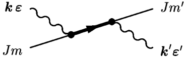
FIG. 2. Feynman diagram for the transition-matrix element T_{fi} [Eq. (8)] near resonance. Wavy lines denote photons, straight lines atomic internal states. The thick line stands for the dressed propagator (\delta + i\Gamma/2)^{-1} of the excited atomic state. The absorption vertex yields a factor \omega_R \exp(i\mathbf{k} \cdot \mathbf{r}) \langle J_e m_e | \boldsymbol{\epsilon} \cdot \mathbf{d} | Jm \rangle , the emission vertex yields a factor \omega_R \exp(-i\mathbf{k}' \cdot \mathbf{r}) \langle Jm' | \bar{\boldsymbol{\epsilon}}' \cdot \mathbf{d} | J_e m_e \rangle , and all intermediate variables, here m_e , have to be summed over.
