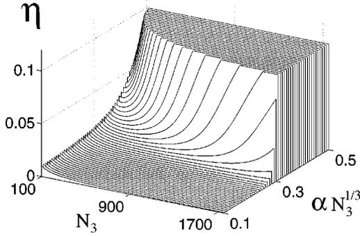
FIG. 2. Analytical estimate of the Bragg process efficiency. The model is limited by the assumption  $\eta \ll 1$ . For small values of  $\alpha$ , the efficiency decreases with increasing  $N_3$ .
