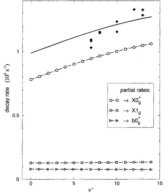
FIG. 3. Calculated partial (dashed lines) and total (solid line) radiative decay rates of  $A0_u^+, v'$  states of  $Te_2$  ( $J'=50$ ) as functions of the vibrational quantum number. Experimental collisionless lifetimes (Ref. [17]) for  $J'=50 \pm 5$  are marked by filled diamonds.
