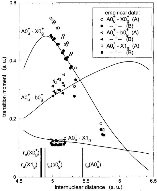
FIG. 2. *Ab initio*  $A0_u^+ \rightarrow X0_g^+, X1_g, b0_g^+$  transition dipole moment functions (solid lines) and empirical transition moment estimates as functions of  $r$  centroids [16] [A, empty symbols: original normalization corresponding to  $\tau(A0_u^+, v'=11) = 670$  ns; B, filled symbols: values renormalized to  $\tau(A0_u^+, v'=11) = 844$  ns [17]].
