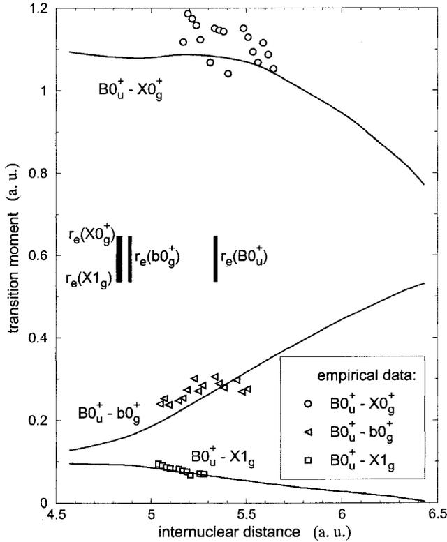
FIG. 4. *Ab initio*  $BO_u^+ \rightarrow X0_g^+, X1_g, b0_g^+$  transition dipole moment functions (solid lines) and empirical transition moment estimates from Ref. [16].
