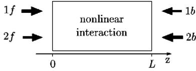
FIG. 1. Four matter waves incident into a region of nonlinear interaction. The two forward moving and the two backward propagating modes, with opposite wave vectors, are distinguished by their internal state.
