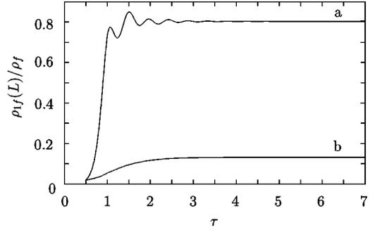
FIG. 5.  $\rho_{1f}(L, \tau)$ , normalized to  $\rho_f$ , for  $\rho_{1f}(0)=0.01\rho$ . The time is in units of the round-trip time through the interaction medium. Curve (a) is in the regime with only one high-output stable branch at  $L/L_c=4\pi$ ; curve (b) is at  $L/L_c=1.6\pi$  where for every (low) output intensity there exists a stable steady-state field configuration.
