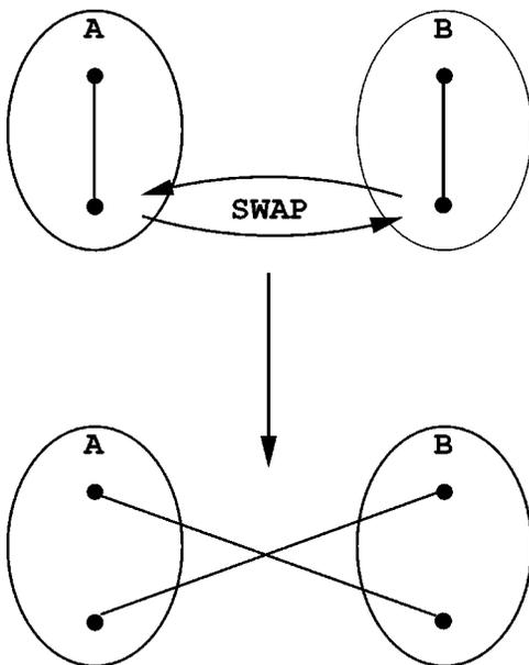
FIG. 3. Illustration of how the SWAP operation can be used to establish two ebits of entanglement between A and B.
