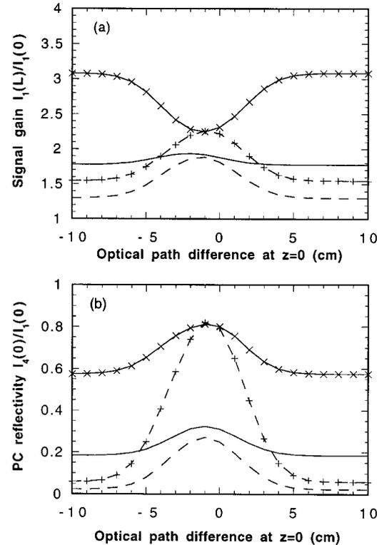
FIG. 2. Signal gain and the PC reflectivity as a function of the optical path difference between the signal beam and the second pump beam at position  $z=0$ . Solid lines are for the transmission grating dominated case (case 1), broken lines are for the reflection grating dominated case (case 2). The curves with (without) symbols are for  $\beta = 100$  ( $\beta = 1$ ), respectively. (a) Signal gain; (b) PC reflectivity.
