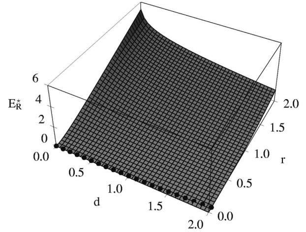
FIG. 2. The upper bound  $E_R^*$  for the relative entropy of entanglement of the state of Eq. (17) as a function of the squeezing parameter  $r$  and the degree of damping  $d(=\gamma t)$ . The averaged number of photons in the thermal environment  $\bar{n}=0.01$ . The dotted line is the separability-inseparability borderline. The amount of  $E_R^*$  is shown in units of bits.
