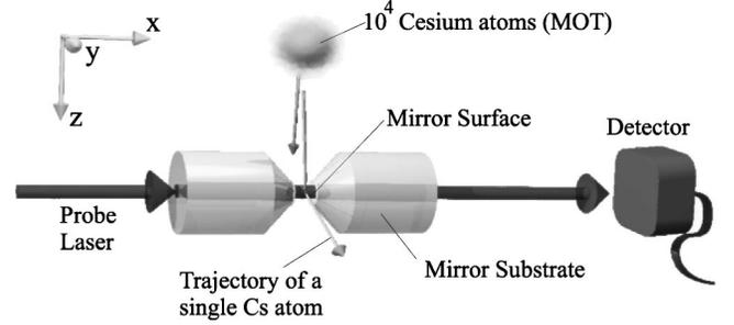
FIG. 2. Experimental schematic for the case of Hood *et al.* Atoms are captured in a magneto-optical trap (MOT), and dropped or launched through a high-finesse optical cavity. A single atom (trace with arrow) transiting the cavity mode alters the measured transmission of a probe beam through the cavity. In the experiment of Pinkse *et al.*, rubidium atoms are captured in a MOT below the cavity and launched upward through it.
