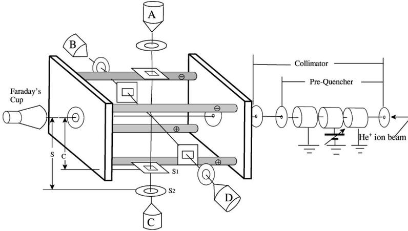
FIG. 2. Schematic diagram of the apparatus for the  $\text{He}^+$  anisotropy measurements. The four metal rods in the observation cell are 1.2700(2) cm in diameter and are supported 4.064(1) cm apart on insulators.  $S_1$  and  $S_2$  are photon collimating slits with  $c=7.117(2)$  cm and  $s=21.999(3)$  cm. Details of the schematically drawn photon detectors  $A, B, C,$  and  $D$  are shown in Fig. 3 below.
