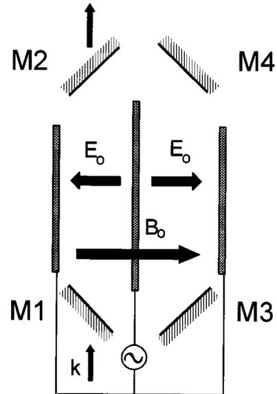
FIG. 2. Proposed geometry to increase the effective optical path length for a determination of the magnetoelectric Jones birefringence.  $M1$  and  $M2$  should be highly reflecting, slightly transmitting mirrors, and  $M3$  and  $M4$  should be 100% reflecting mirrors.
