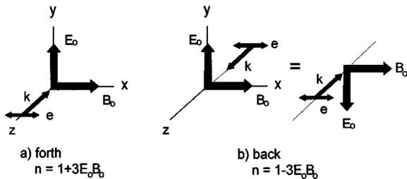
FIG. 1. Schematic view of the properties of the magnetoelectric linear birefringence in multipass cavities. The magnetoelectric effects on the refractive index on forth and back passages are shown to be opposite. A similar conclusion holds for magnetoelectric Jones birefringence. We have omitted the Cotton-Mouton and Kerr contributions for clarity.
