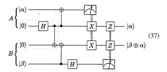
The prohibited operation in the dotted box is applied to a known state, and can be replaced by the EPR state of Eq. (32). Provided such a shared entangled state is initially available to Alice and Bob, they can perform a remote CNOT operation using two bits of classical communication.
