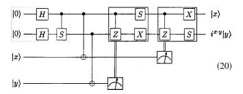
where the double lines control all the operations in the corresponding boxes. All the circuit elements in Eq. (20), except those in the dotted box, can be performed fault-tolerantly. Finally, we can replace the dotted box by an input ancilla in the following state:
