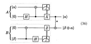
The prohibited CNOT gate can be commuted backwards to obtain a remote CNOT circuit:
