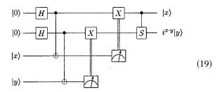
Commutating  $\Lambda_1(S)$  backwards using the commutation rules in Eqs. (17) and (18), we obtain a circuit for the controlled-phase gate:
