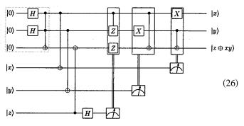
All the circuit elements except those in the dotted box can be performed fault-tolerantly. It remains to prepare the state created in the dotted box,
