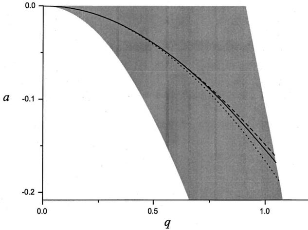
FIG. 3. Section of the stability diagram for the harmonic linear Paul trap (gray-shaded area). The curves represent the borderline for two-ion crystals being oriented along the  $z$  axis for the simplified pseudopotential given by Eq. (7) plus a  $1/\rho$  Coulomb term (dotted line), for the pseudopotential given by Eq. (12) (dashed line), and from molecular dynamics simulations (solid line). Above the lines, the two-ion crystal is supposed to be oriented along the  $z$  axis.
