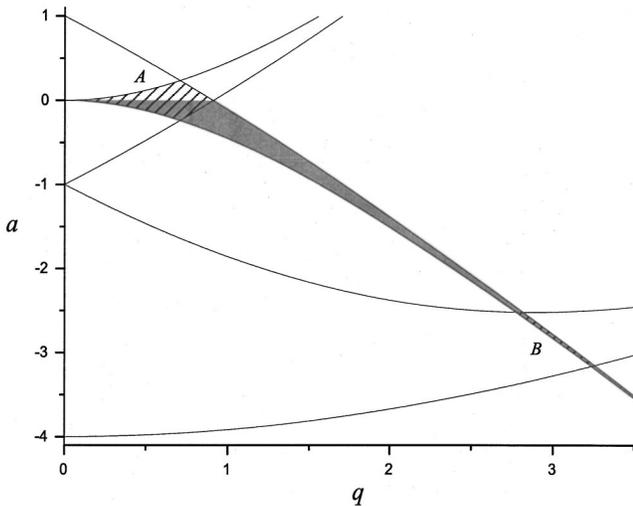
FIG. 2. Single-ion stability diagrams for the quadrupole mass filter (the hatched areas  $A$  and  $B$ ) and for the harmonic linear Paul trap (gray-shaded area). The dimensionless parameters  $a$  and  $q$  are defined in the text.
