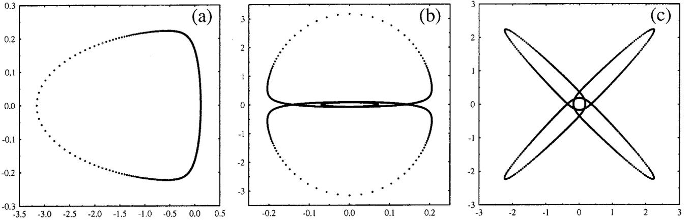
FIG. 2. Closed orbits of a particle in the screened 2D isotropic harmonic oscillator of Eq. (12), with  $\lambda=0.2$  and  $E=5$ . (a)  $\kappa=1/2$ , (b)  $\kappa=1/3$ , and (c)  $\kappa=2/3$ .
