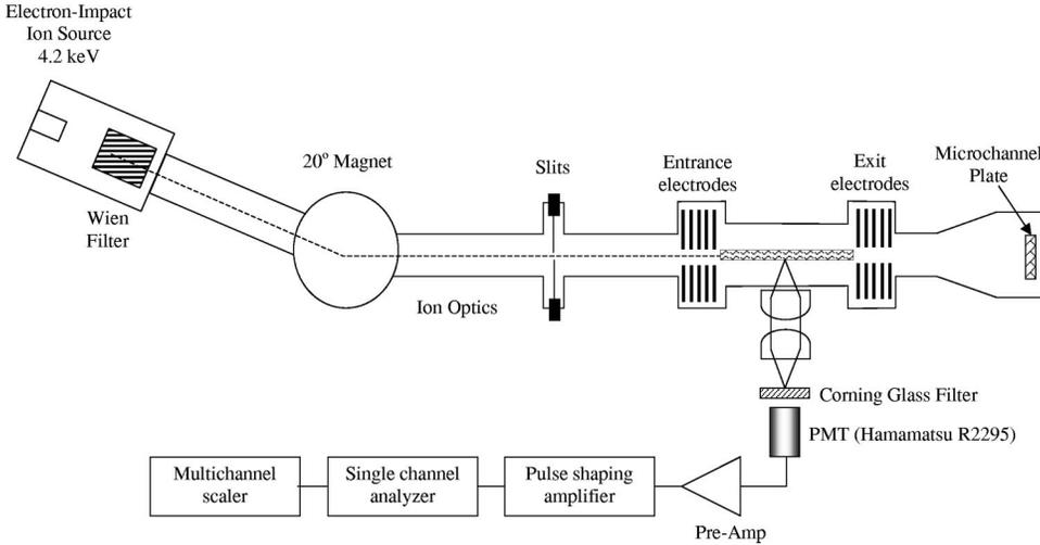
FIG. 1. Schematic of the experimental setup with the photon counting system.
