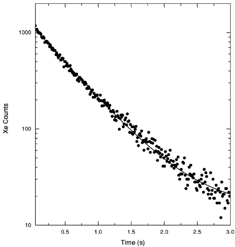
FIG. 3. Neutral and singly charged Xe atoms signal from the microchannel plate detector as a function of time. The solid line is the fit to the data as described in the text.
