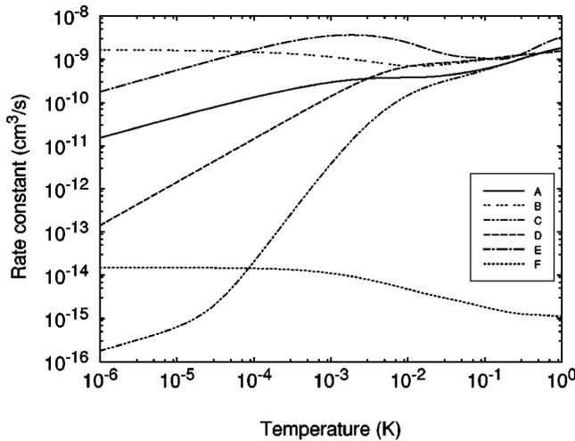
FIG. 1. Elastic and ionization loss rate constants as a function of temperature for various transitions: (A)  $j=0 \rightarrow j=0$ , (B)  $j=0 \rightarrow PI$ , (C)  $j=1 \rightarrow j=1$ , (D)  $j=1 \rightarrow PI$ , (E)  $j=2 \rightarrow j=2$ , and (F)  $j=2 \rightarrow PI$ .
