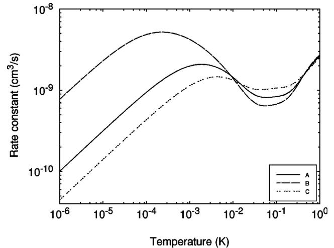
FIG. 2. Total elastic rate constant as a function of temperature for (A) no variation, (B) +1%, and (C) -1% variation of the short-range  $^5V_\Sigma(R)$  potential.
