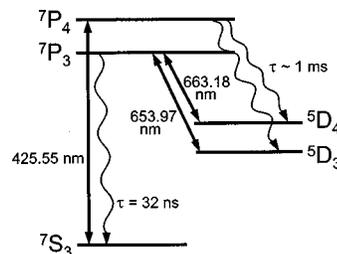
FIG. 1. Energy-level diagram for chromium, showing the principal laser cooling transition, the ‘‘optical leaks,’’ and the repumping transitions.
