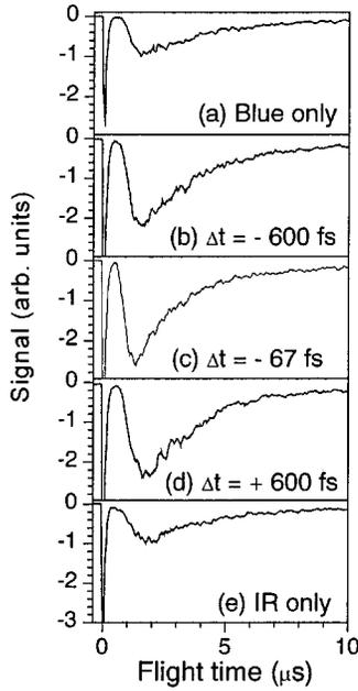
FIG. 2. Measured ion time-of-flight spectra from the irradiation of 14 000-atom Xe clusters with a 780-nm and/or 390-nm laser pulse. (a) Blue pulse only. (b) Blue precedes IR by 600 fs. (c) Blue precedes IR by 67 fs. (d) Blue pulse 600 fs after IR. (e) IR pulse only. In each case the intensity of the 780-nm pulse was  $6 \times 10^{14} \text{ W cm}^{-2}$  and that of the 390-nm pulse was  $2.5 \times 10^{15} \text{ W cm}^{-2}$ .
