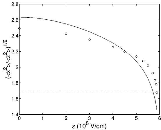
FIG. 4. Electric-field dependence of the width aspect ratio for parameters of Fig. 2. The solid line is the result of our variational calculation while circles denote exact numerical results. The dashed line corresponds to  $\sqrt{\langle x^2 \rangle / \langle z^2 \rangle} = \sqrt{8}$ , for a noninteracting gas in a TOP trap.
