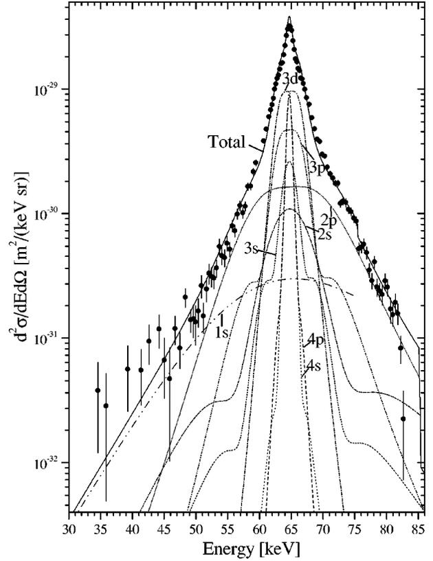
FIG. 4. The experimental values of the differential cross section  $d^2\sigma/d\Omega dE$  for Compton scattering in germanium and the theoretical values calculated using the impulse approximation with the hydrogenlike wave functions.
