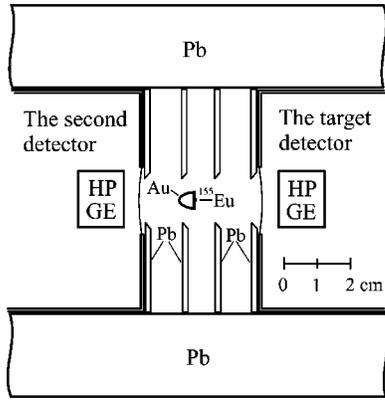
FIG. 1. A part of the experimental setup for the coincidence measurement of the Compton spectrum.
