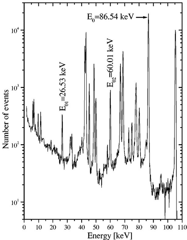
FIG. 2. The spectrum of  $^{155}_{63}\text{Eu}$  measured in the target detector. The Compton spectrum was determined for the 86.54-keV  $\gamma$  rays.
