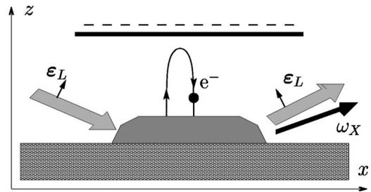
FIG. 1. Sketch of the Farkas and Horváth experimental setup. The laser pulse shining at grazing incidence on a gold target creates a surface plasma. Energetic electrons, which normally escape from the plasma, are pushed back by a constant negative voltage and recombine with ions generating at the same time x-ray radiation.
