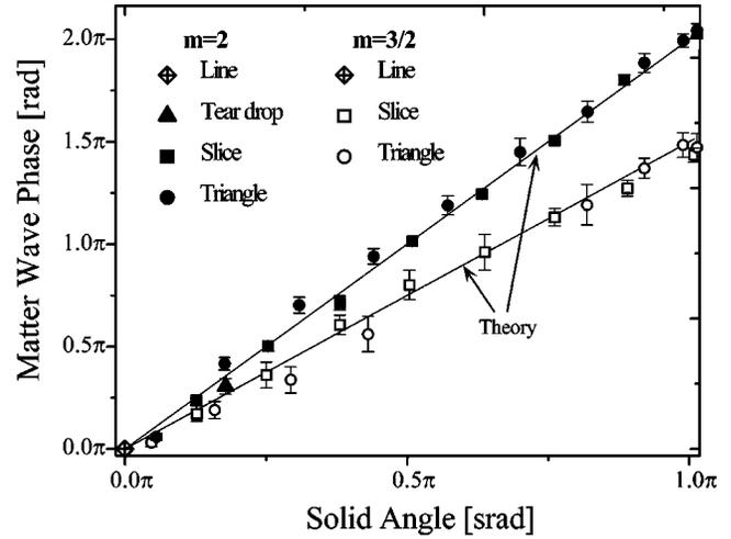
FIG. 4. Summary of the experimentally determined geometric phases as a function of the solid angle  $\Omega$ . Systems with effective spins equal to  $3/2$  (open points) and  $2$  (solid points) are displayed for the four types of paths shown in Fig. 2. The solid lines are plots of the equation  $\gamma = m\Omega$ , where  $m$  is the corresponding maximum magnetic quantum number for the spin.
