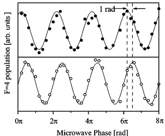
FIG. 1. Fringes from the adiabatic transfer (AT) atom interferometer. In the first set of data the interferometer used two identical AT pulses, while the second set shows data obtained when the phase difference between the AT beams is changed during the final pulse. The phase difference was altered in a way such that the starting and finishing values were the same. Note that the fringes in the two experiments are shifted with respect to each other by approximately 1 rad. This is a Berry phase.
