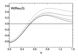
FIG. 7. Simulations for a cross section of the Wigner distribution when the velocity distribution is Gaussian. The solid line represents the true Wigner function for a Fock state with n=1, while the dashed, dash-dotted, and dotted lines are simulations for  $M\Delta v_x$ equal to  $0.025h/\lambda$ ,  $0.050h/\lambda$ , and  $0.10h/\lambda$ .  $G^2 t_{int}/\Delta = \pi$ .
