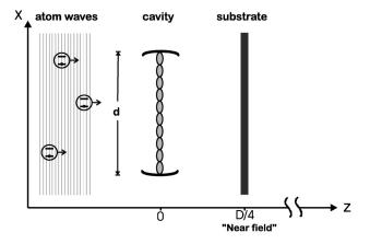
FIG. 1. Two-level atoms coming from the left interact with the field in the cavity and are detected on a substrate at z=D/4.
