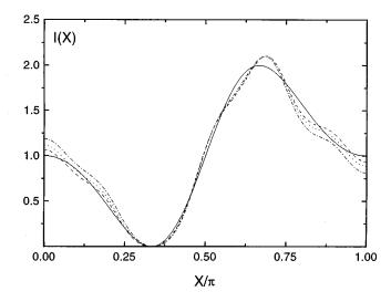
FIG. 3. Intensity I(X) at z=D/4 for (a) infinite aperture (solid line); (b)  $a=10\lambda$ ,  $\eta=0$  (dashed line); (c)  $a=10\lambda$ ,  $\eta=0.04$  (dotted line); (c)  $a=10\lambda$ ,  $\eta=0.10$  (dash-dotted line).
