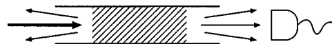
FIG. 1. Coherent light (thick arrow) is incident on an amplifying medium (shaded), embedded in a waveguide. The transmitted radiation is measured by a photodetector.
